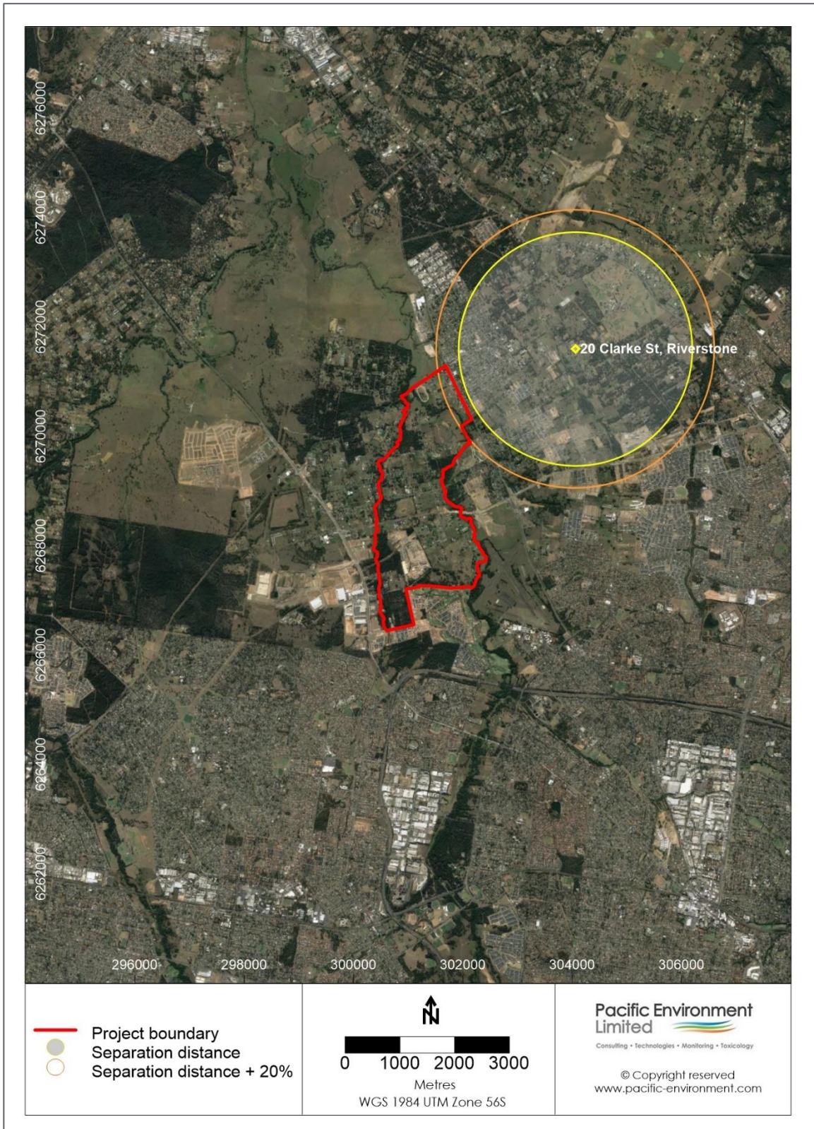
Figure 3.9: Level 1 separation distance for broiler farm at 20 Clarke Street, Riverstone
